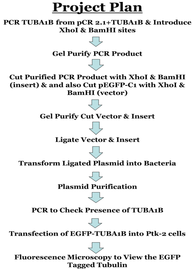
Figure 7: A flow chart depicting the steps the students will follow to create the original pEGFP-tubulin-6 construct.
