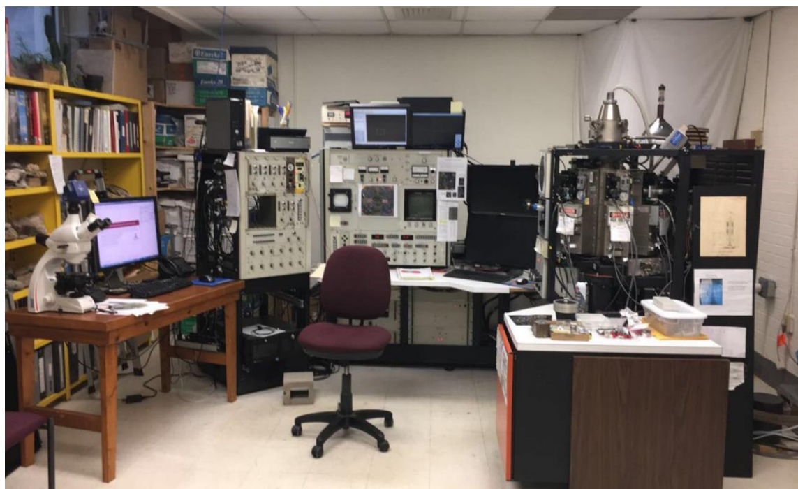
Figure 4: Concord University's ARL-SEM electron microprobe, used for chemical analysis of tephra samples.
