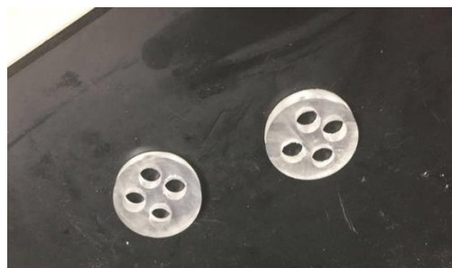
Figure 3: Example of mounts used for tephra samples before placing them in the microprobe.
